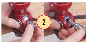
Just push the button and remove the metering insert.
